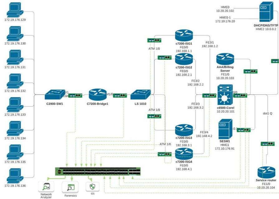
**Use Case:** TAP 8 links in different locations and aggregate down to one monitoring port.
