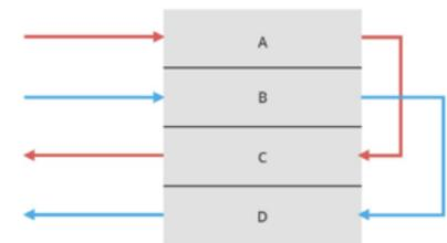
This diagram depicts a 4 port (A, B, C, D). The Data Diode SPAN TAP shows the traffic of portA flow out of portC and PortB flow out of PortD.
