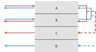
This diagram depicts a 4 port (A, B, C, D). The Data Diode Network TAP shows portA flow out of portB, and sends a copy out of portC and PortB flow out of PortA, and sends a copy out of portD.
