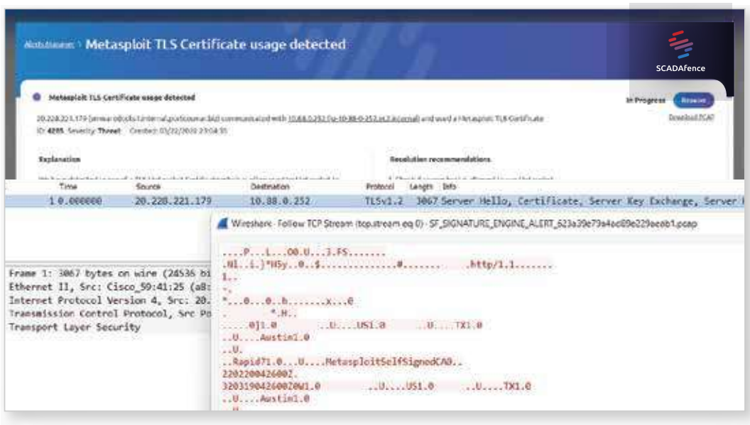
Detecting a Metasploit Certificate Usage. Every alert includes the PCAP file to help further investigate the issue.
